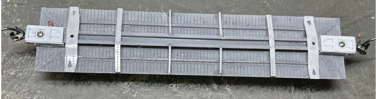
Photo shows the couplers, cross-ties and bearer and bolster caps. The B end has been marked.
