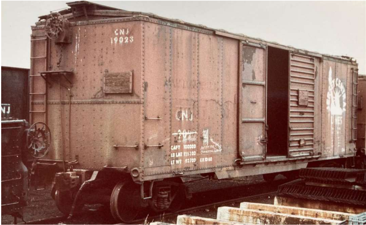
CNJ 19023 circa early 1960s. Note lined out number indicating no longer in revenue service, and original half door.
