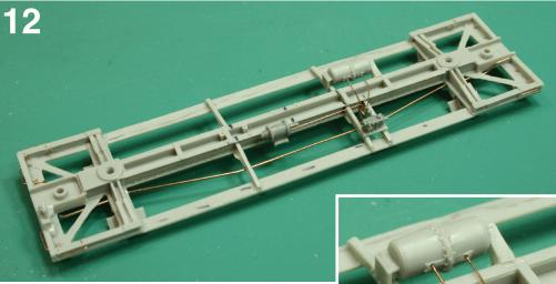
plate's bottom edge rests on the horizontal reservoir support just added. The reservoir is 24" from the center of the center sill. Position the reservoir on the two supports with the two lugs towards the "B" end and the air pipe ports facing inward. Fix in place [Photos 9, 10, 11, 12].
