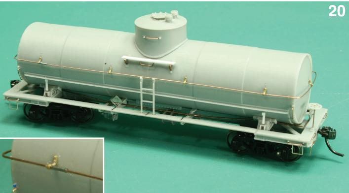
There will be two pieces, with each running down one side of the tank to the wide stanchion and including one curved end. Trim the ends of the pieces so that the ends of each meet within the wide stanchions. Fix the wire ends inside the wide stanchion castings with glue. Soldering with a low wattage iron also works. Straighten the handrails as necessary by adjusting the angle of the stanchions.
