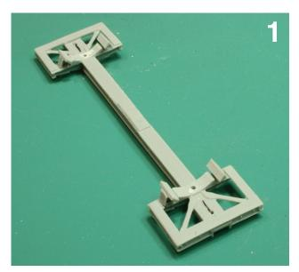
each end of the underframe platform and from the top of the center sill as these are casting vents. Do not remove the raised rectangular pad from the top of the center sill as this locates the tank. For this reason, clean the edges of this pad, making sure they are square. Clean and square off the edges of the end platform running boards so there will be a good joint for the long running boards between the platforms [Photo 1].
