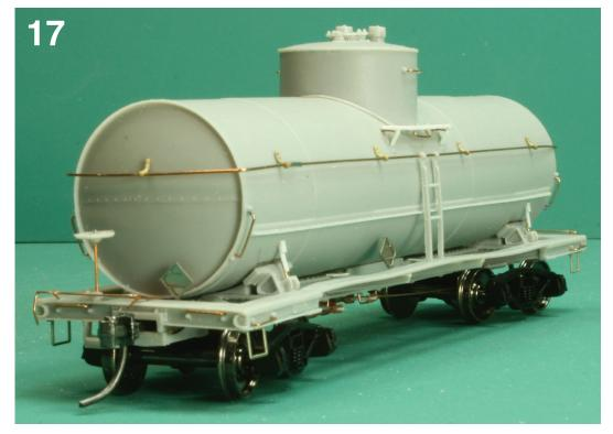
c. Drill for 0.0125" wire and form and install four grabs at the lower tank corners [Photos 17, 19, 20].
