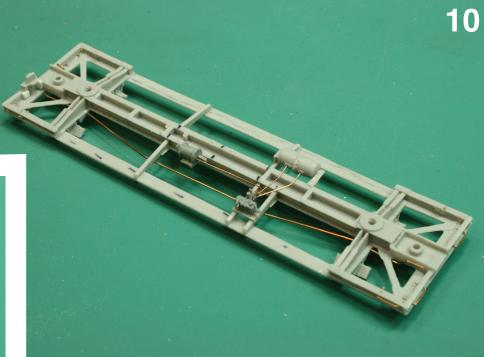
to just behind the AB valve. Add a short piece of wire from the pipe tee to the AB valve [Photos 7 (inset), 8].
