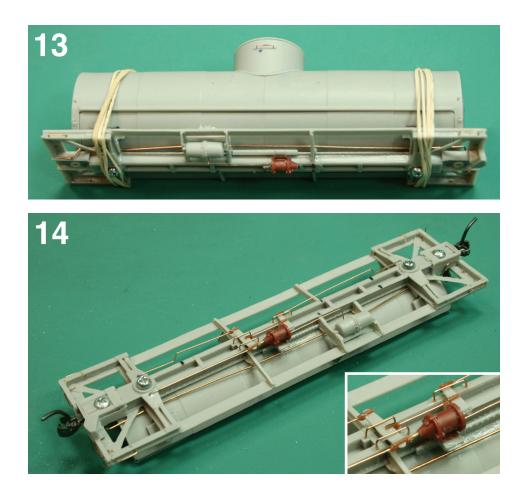
k. Attach the tank band connection gussets to the outside of the saddles. These are the "U" shaped brackets located inside the ladder rungs. Drill #76 holes in the tops of the gussets.
