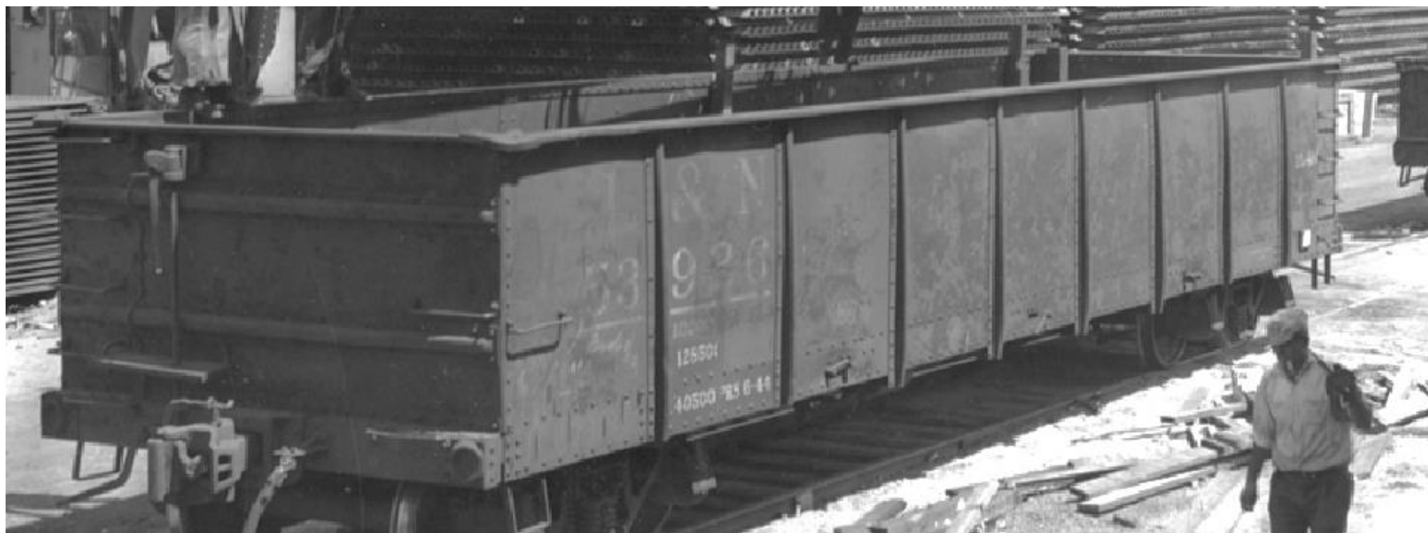
This mid-1940s view of the B end of 53926 shows off the lever hand brake applied to these cars. Bill Welch collection.
