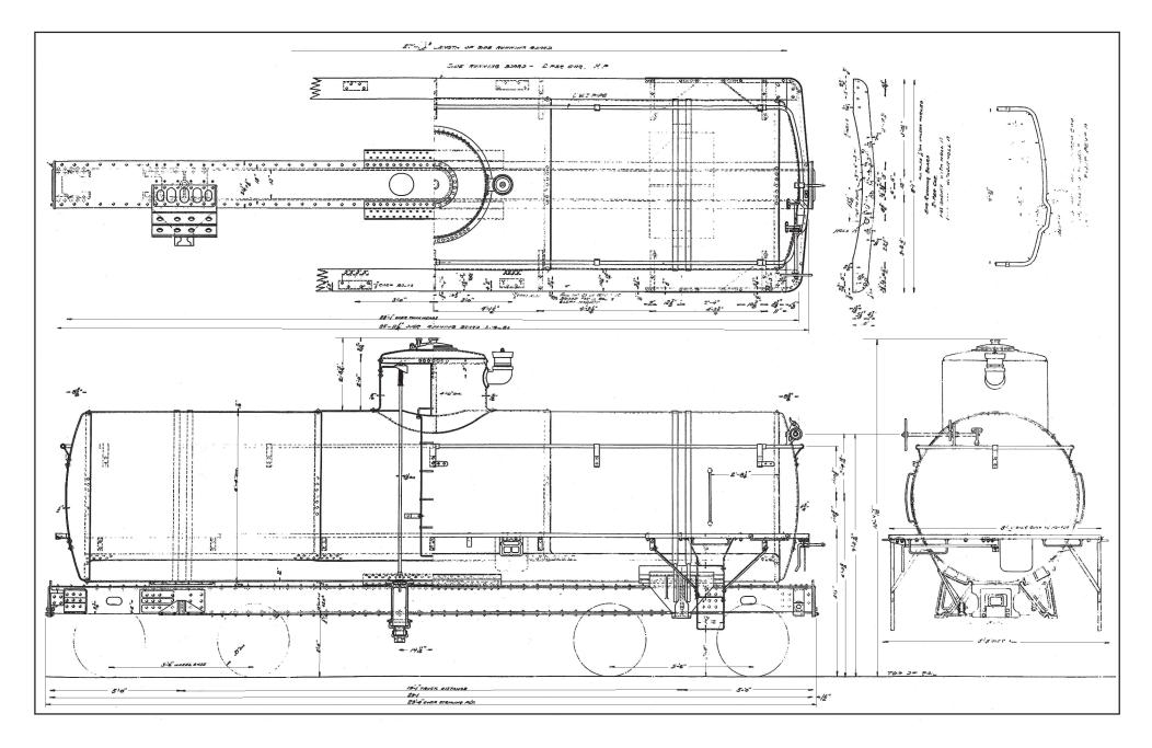
UTLX Class X 6,500 Gallon Tank Car GA Drawing April 22, 1915 Scale: 1/4 inch = 1 foot
