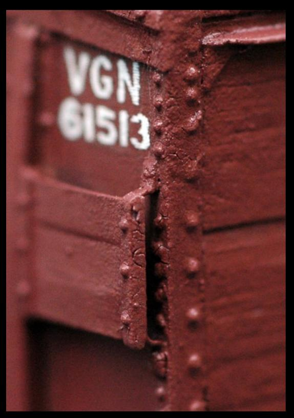
Here is a mounting bracket with a Placard board in place and painted.
