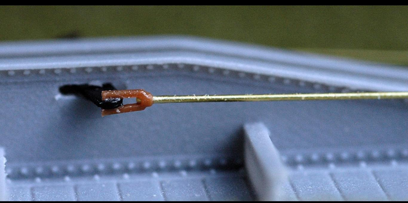
Tichy's styrene turnbuckle makes a good clevis too!
