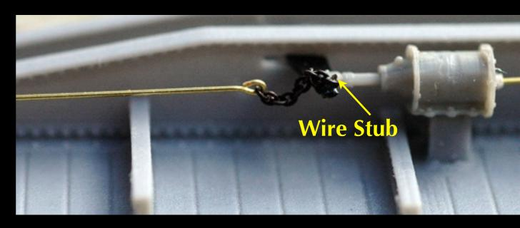
and tease the chain onto it and cut the chain leaving 6-8 loops of chain. With the brake cylinder and lever in place I tease the chain onto the wire stub and secure it with CA.
