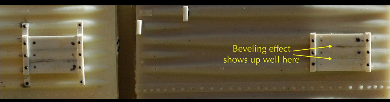
In the case of the IC boxcar, I was also building a Sunshine IC boxcar kit so instead of two Placard Boards I made six. The key in gluing the "boards" down is to make sure a beveled edge abuts a sharp edge. Sometimes I bevel both edges. Boards are glued to a .005 substrate.
