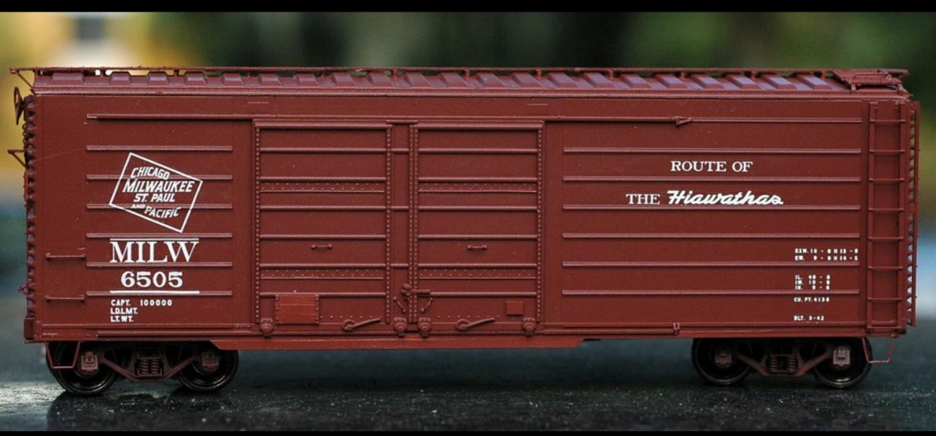
Although there is some compromises along the bottom of the sill that I could not figure out how to solve, the overall result was very pleasing for me. The ladders were scratch built.
