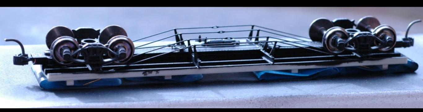
I like to use Brass Wire and Grandt Line Brass Turnbuckles and keep the turnbuckle's center open.
