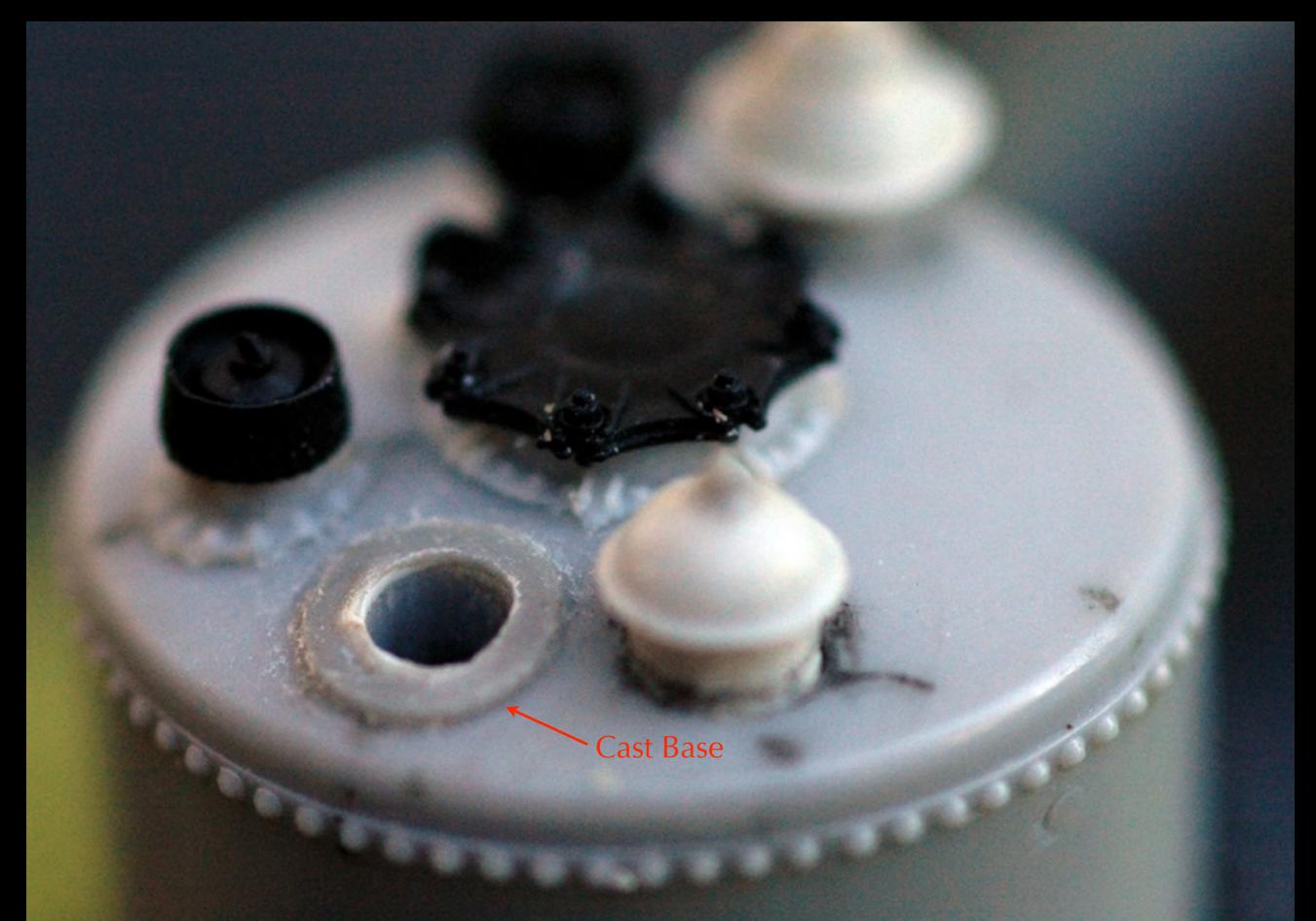
I used CA to add a filet around the base to give it the appearance of being one piece. Almost finished here or so I thought. . .
