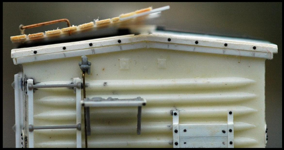
The sheet metal of the Hutchins roof was bent over the very end and riveted or bolted in place. I used a veneer of .010 and .005 styrene and *Athearn* rivets to recreate this look, carefully filing and sanding the edges of the roof to model the look of the bent metal. Note the *Yarmouth* photo-etched eyebolt at the corner of the roof grab.
