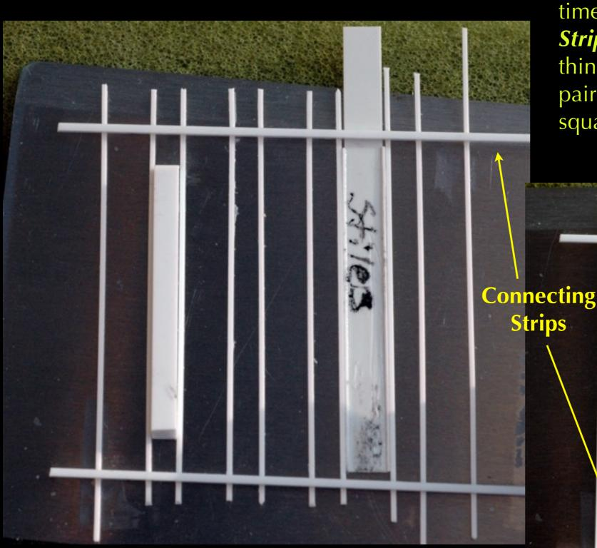
The key is exactly spaced stiles: In place are two styrene *Spacers*. The wider one goes between each pair of stiles as I glue them down one at a time to what I will call the *Connecting Strips* at each extreme end. The thinner Spacer fits between each new pair of stiles keeping everything square and parallel.
