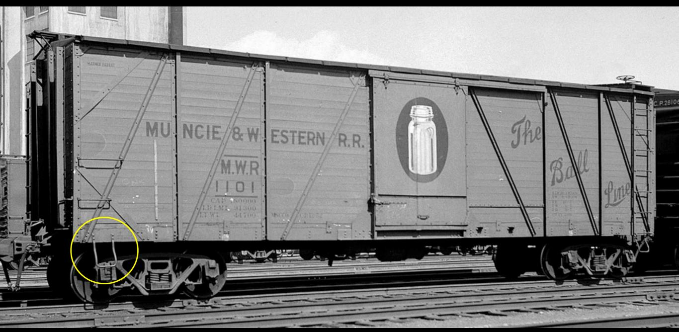
The cars built and leased by the Mather Company used round bars fabricated into Sill Steps and modelers have to do the same thing to model them.
