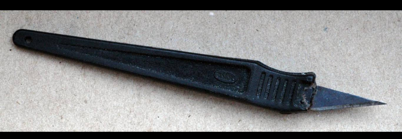
**Dull** Disposable *Testors* Hobby Knife for Placing Rivets
